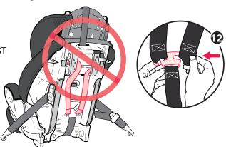
11. Check that the straps are inserted at the same level. Pull on harness to make sure it is secure 13.
